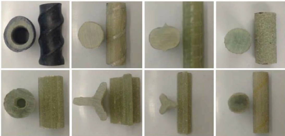
Figure 4 - GFRP rebar with different cross-sectional shapes [9]
